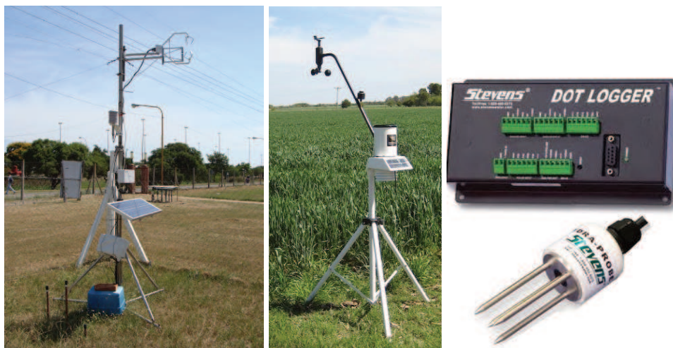
Figure B.18: Eddy covariance station, Pegasus station and Stevens data-logger.
