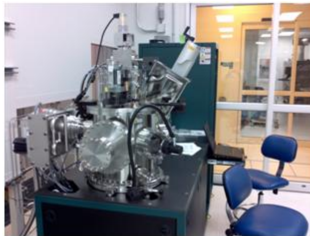
Figure 5.13: AJA ATC Orion thin film deposition system.
