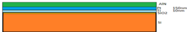
Figure 5.12: Scheme of the heterostructure of AlN/Pt/Ti/SiO 2 /Si.
