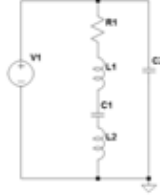
Figure 3.6: Modified Butterworth-Van Dyke equivalent circuit for a surface-loaded piezoelectric resonator.
