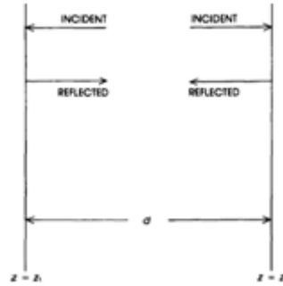
Figure 3.7: Finite thickness acoustic medium: at all points in the medium, there are right and left propagating plane waves. 9
