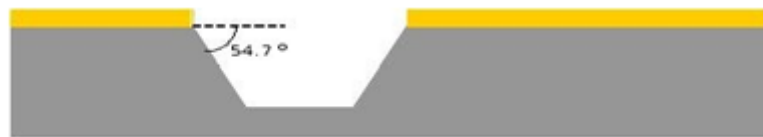
Figure 5.23: Si (100) showing characteristic V anisotropic etch of the walls forming an angle of 54.7^\circ with respect to the main surface.
