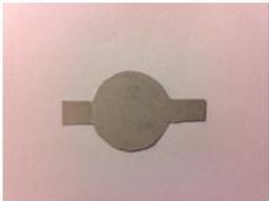
Figure 5.2: Disk-shaped piezoelectric PVDF with silver ink electrodes.
