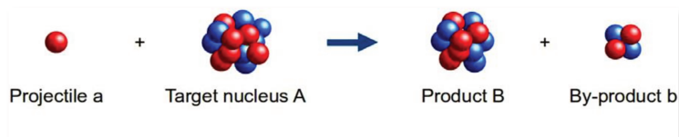
Figure 1: Nuclear reaction where target nucleus A is bombarded with beam particle a, resulting in the product nucleus B.
