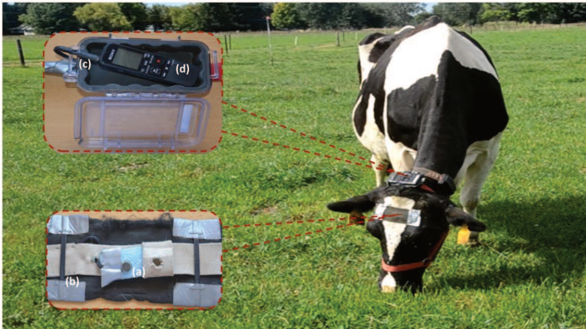
Figure 1. Recording system used to record the acoustic signals composed of inward and outward facing microphones (a). Wired microphones were covered by an elastic headband (b) and plugged (c) into a recorder housed inside a weather proof case attached to the top side of a halter neck strap (d).
