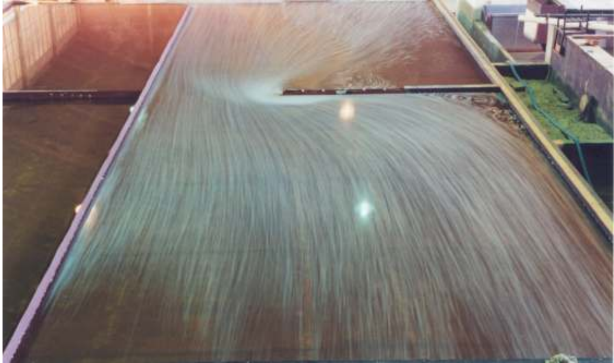
Figure 3.2 Long exposure photograph of the shallow turbulent flow pattern established on a broad experimental basin available at FICH.
