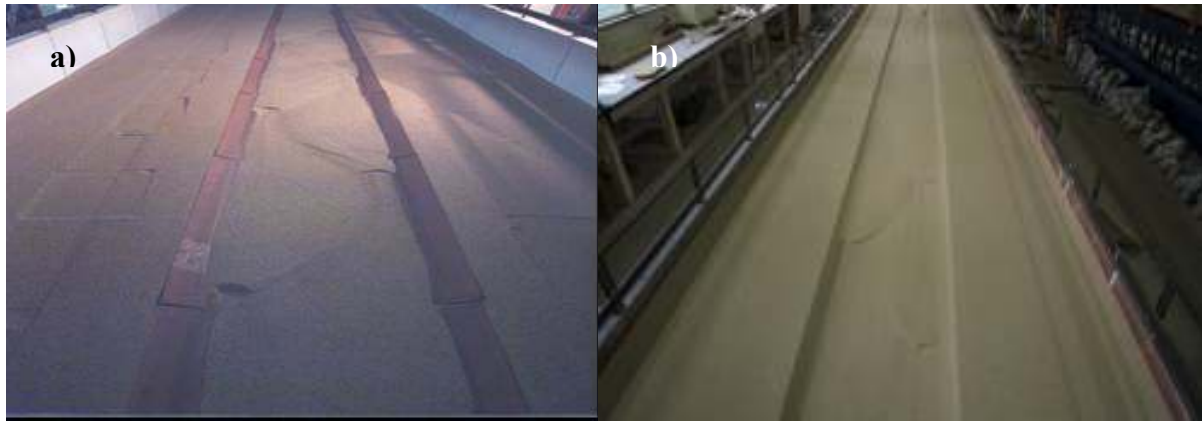
Figure 4.10 a) Experiments with fixed banks; b) Experiments with loose banks.
