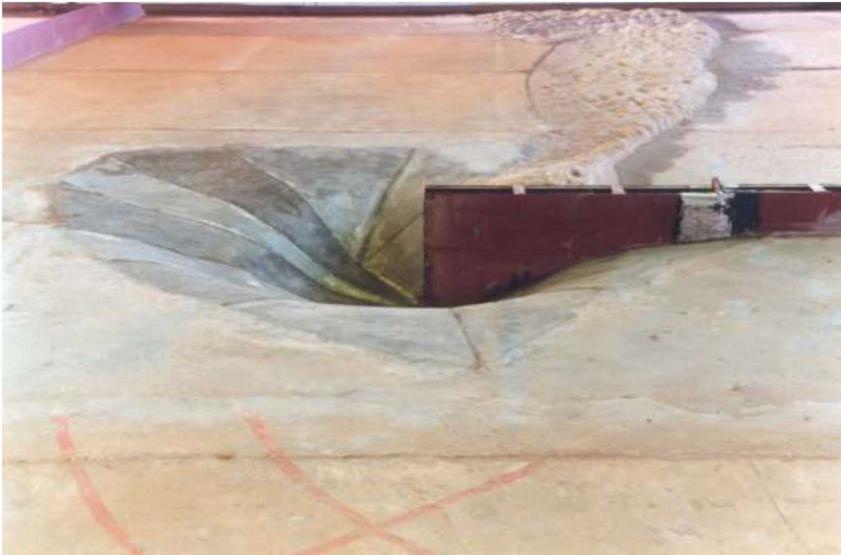
Figure 3.3 Fixed scour hole located at the contraction end.
