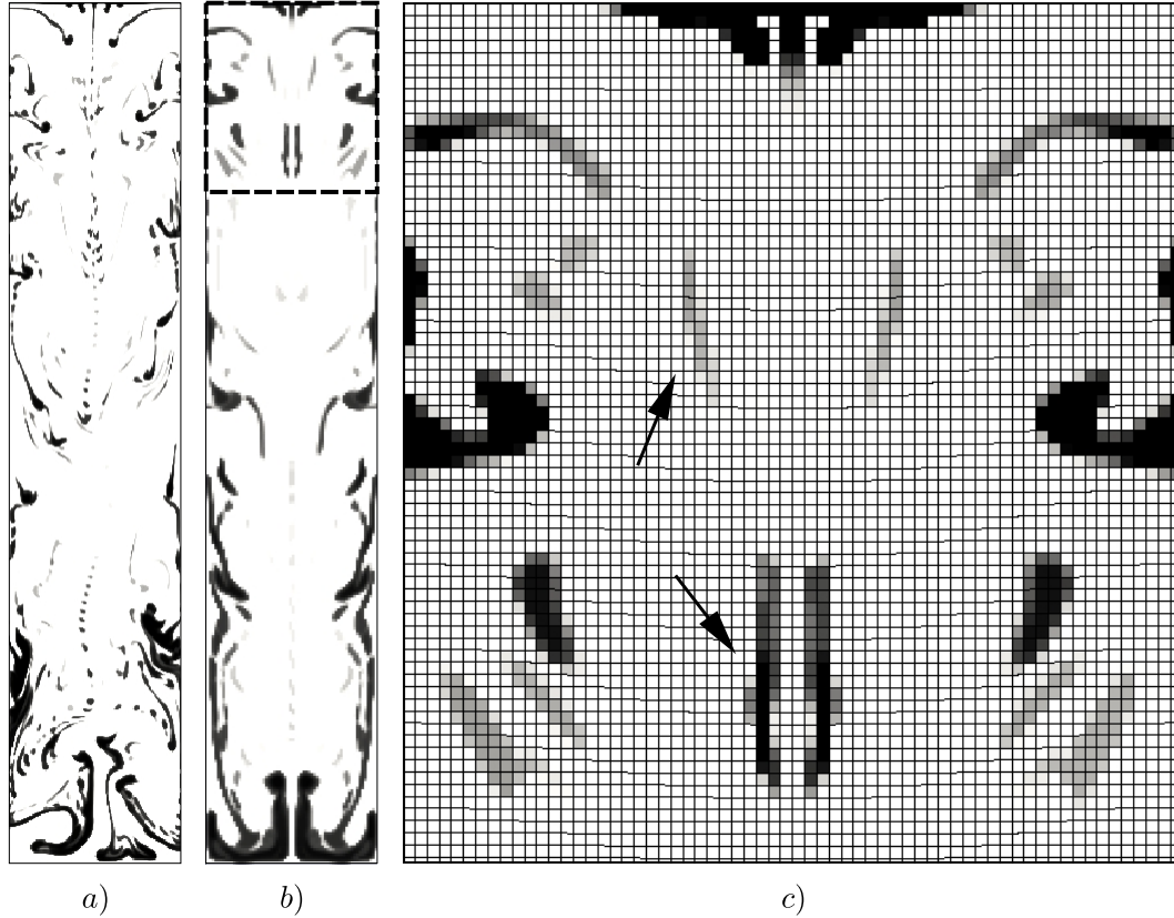
Figure 7.1: Results for the Rayleigh-Taylor problem for t = 5.4 . a) results in fine mesh, b) results in coarse mesh, c) detail for the dashed line box en b) with superimposed mesh (grayscale saturated to black at \alpha_q = 0.3 ). Selected non-resolved chunks are indicated by the arrows.
